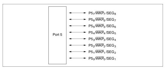
Figure 8.5 Port 5 Pin Configuration
