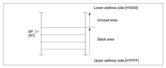
Figure 2.2 Stack Pointer
