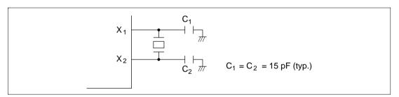
Figure 4.7 Typical Connection to 32.768-kHz Crystal Oscillator
