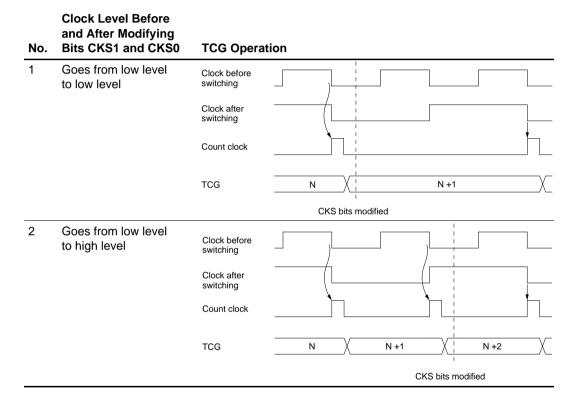
**Table 9.17 Internal Clock Switching and TCG Operation**
