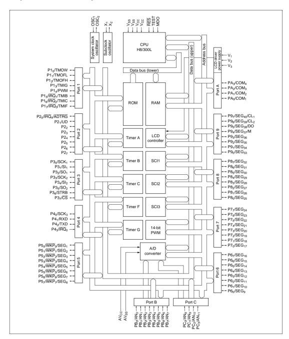
Figure 1.1 Block Diagram
