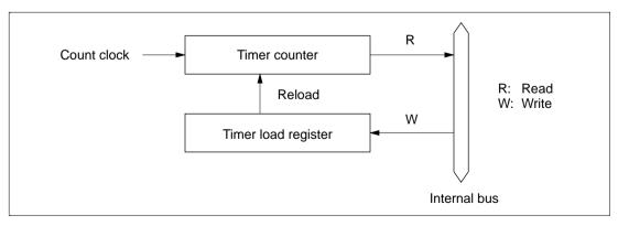
Figure 2.23 Timer Configuration Example
