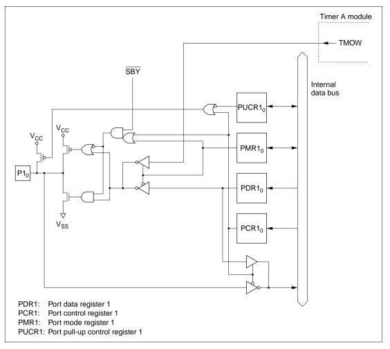
Figure C.1 (e) Port 1 Block Diagram (Pin P1<sub>0</sub>)
