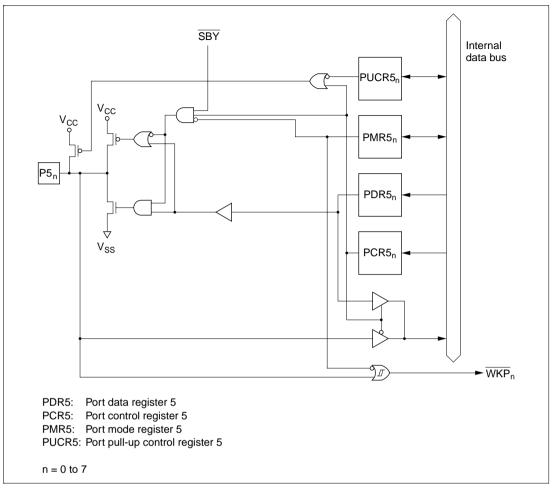
Figure C.5 Port 5 Block Diagram
