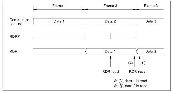
Figure 10.28 Relationship between Data and RDR Read Timing
