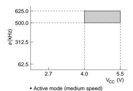
3. Analog power supply voltage vs. A/D converter operating range of H8/3833 and H8/3834
