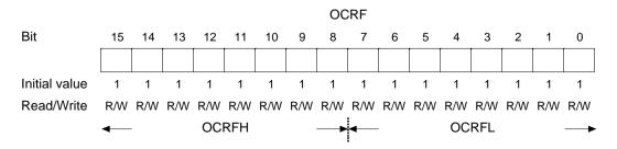
OCRF is a 16-bit read/write output compare register consisting of two 8-bit read/write registers OCRFH and OCRFL. It can be used as a 16-bit output compare register, with OCRFH as the upper 8 bits and OCRFL as the lower 8 bits of the register, or OCRFH and OCRFL can be used as independent 8-bit registers.
