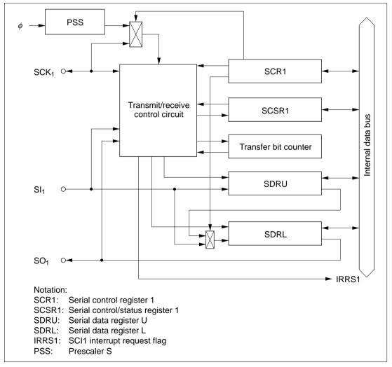
Figure 10.1 SCI1 Block Diagram
