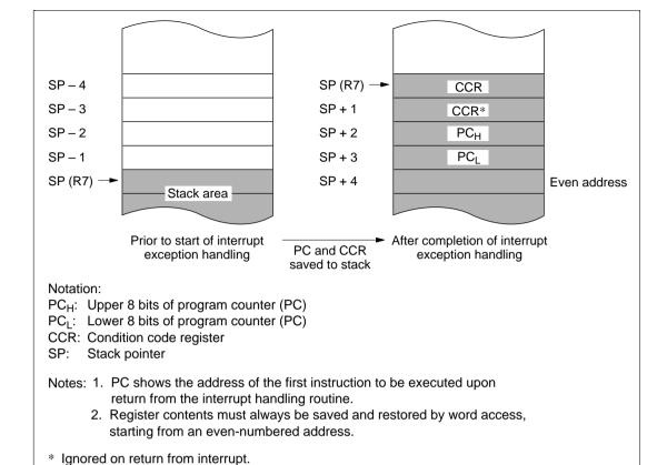
Figure 3.5 Stack State after Completion of Interrupt Exception Handling
