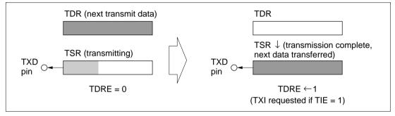
Figure 10.8 (b) TDRE Setting and TXI Interrupt
