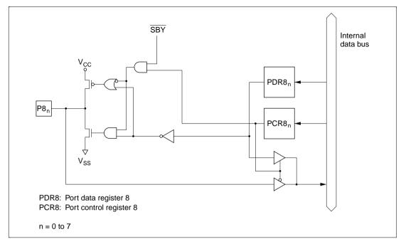
Figure C.8 Port 8 Block Diagram
