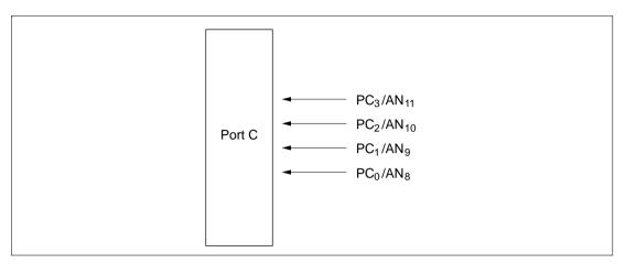
Figure 8.12 Port C Pin Configuration
