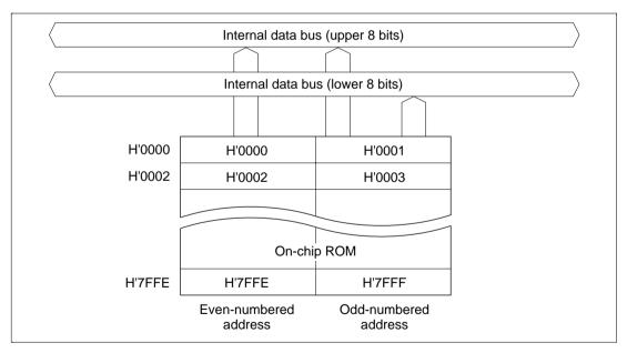
Figure 6.1 ROM Block Diagram (H8/3834)
