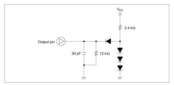
Figure 14.10 Output Load Condition
