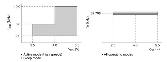
2. Power supply voltage vs. clock frequency range of H8/3835S, H8/3836S, and H8/3837S
