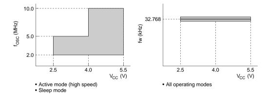
2. Power supply voltage vs. clock frequency range of H8/3832S, H8/3833S and H8/3834S
