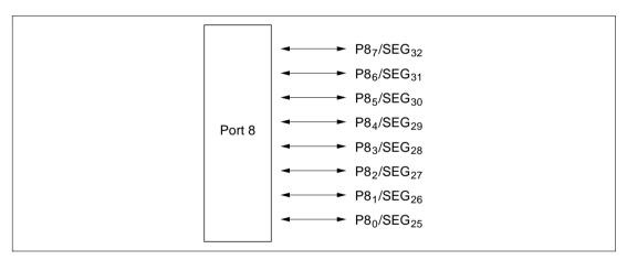
Figure 8.8 Port 8 Pin Configuration
