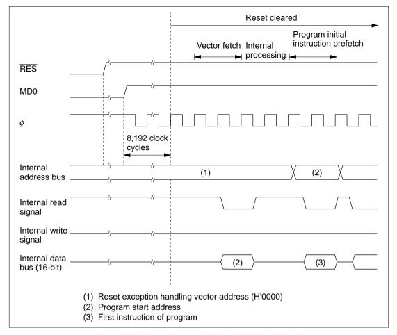
Figure 3.2 Reset Sequence (when MD0 Pin is Low)
