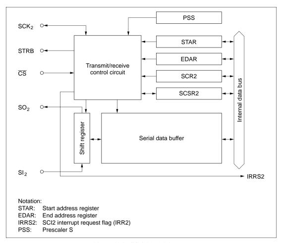
Figure 10.3 SCI2 Block Diagram
