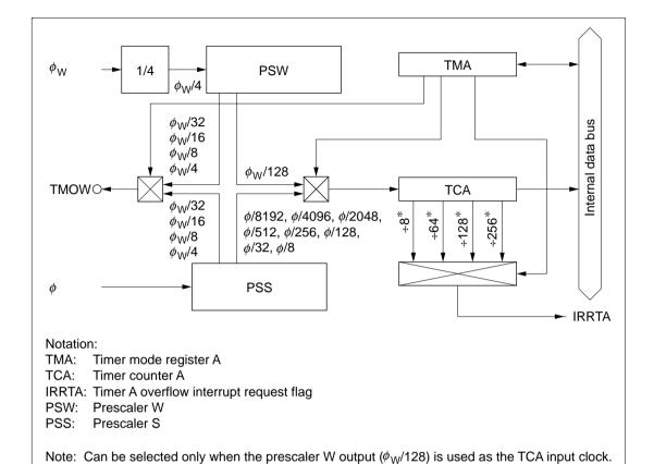
Figure 9.1 Block Diagram of Timer A
