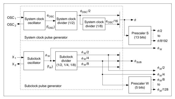
Figure 4.1 Block Diagram of Clock Pulse Generators
