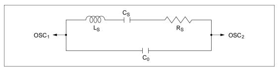
Figure 4.3 Equivalent Circuit of Crystal Oscillator
