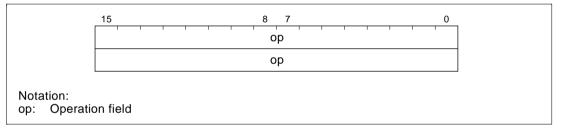
Figure 2.10 Block Data Transfer Instruction Code
