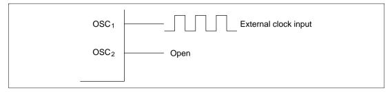
Figure 4.6 External Clock Input (Example)
