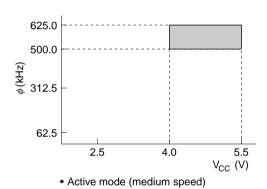
3. Analog power supply voltage vs. A/D converter operating range of H8/3832S, H8/3833S and H8/3834S
