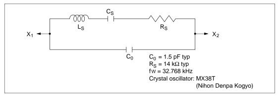
Figure 4.8 Equivalent Circuit of 32.768-kHz Crystal Oscillator
