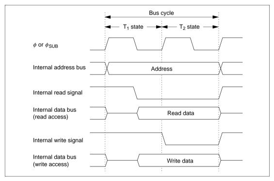
Figure 2.11 On-Chip Memory Access Cycle
