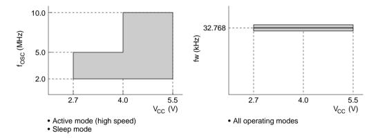
2. Power supply voltage vs. clock frequency range of H8/3835, H8/3836 and H8/3837
