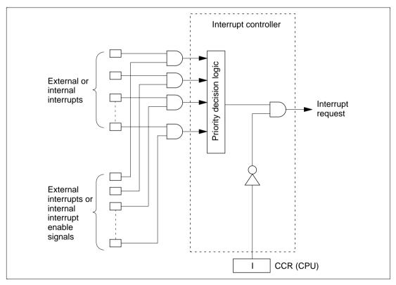
Figure 3.3 Block Diagram of Interrupt Controller
