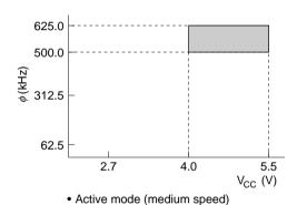
3. Analog power supply voltage vs. A/D converter operating range of H8/3835, H8/3836 and H8/3837
