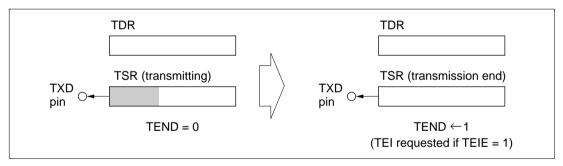
Figure 10.8 (c) TEND Setting and TEI Interrupt
