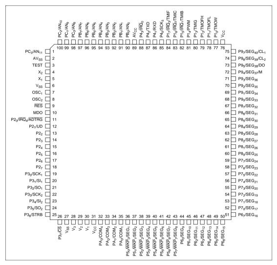
Figure 1.2 Pin Arrangement (FP-100B, TFP-100B: Top View)
