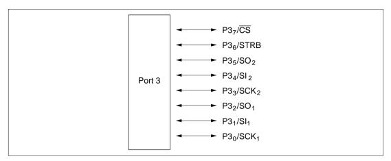
Figure 8.3 Port 3 Pin Configuration
