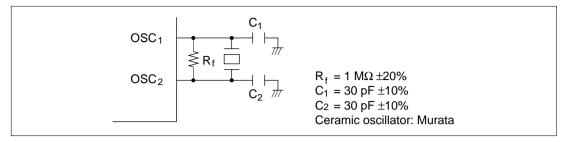
Figure 4.4 Typical Connection to Ceramic Oscillator
