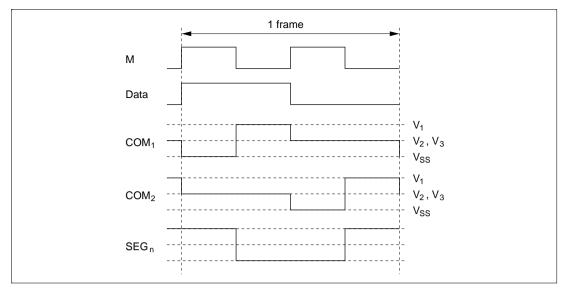
Figure 13.13 (c) Waveforms at 1/2 Duty
