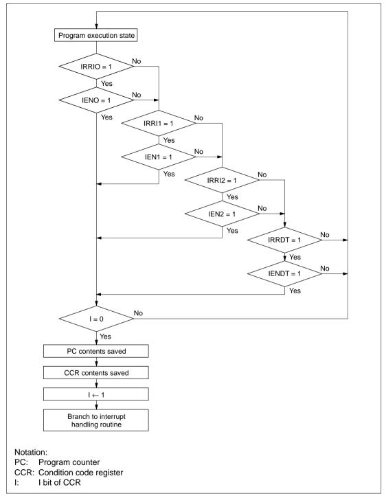
Figure 3.4 Flow up to Interrupt Acceptance
