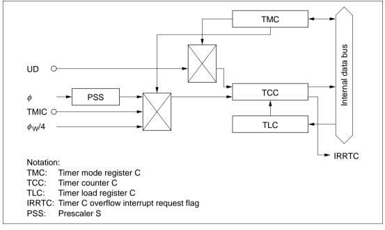
Figure 9.3 Block Diagram of Timer C
