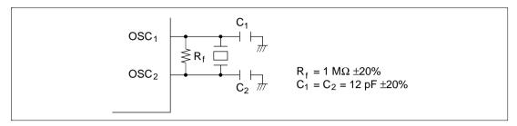
Figure 4.2 Typical Connection to Crystal Oscillator
