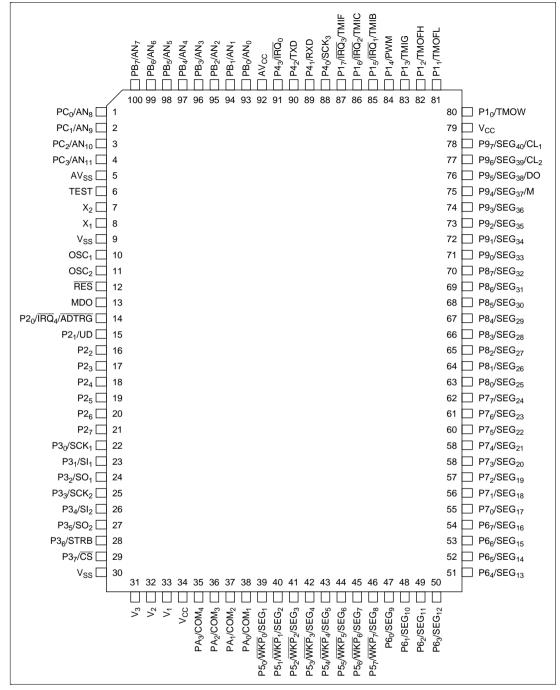
Figure 1.3 Pin Arrangement (FP-100A: Top View)
