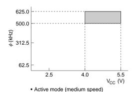
3. Analog power supply voltage vs. A/D converter operating range of H8/3835S, H8/3836S, and H8/3837S
