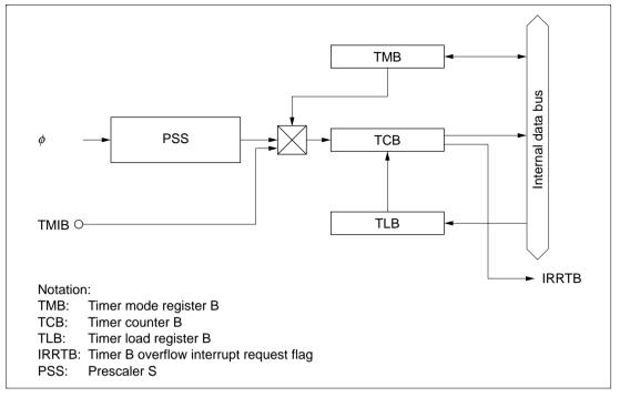
Figure 9.2 Block Diagram of Timer B
