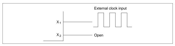
Figure 4.9 Example of Connection when Inputting an External Clock
