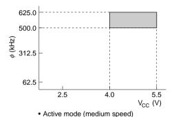
3. Analog power supply voltage vs. A/D converter operating range
