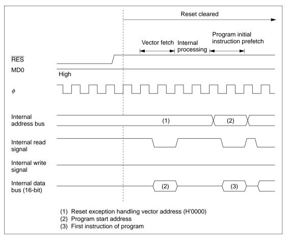
Figure 3.1 Reset Sequence (when MD0 Pin is High)
