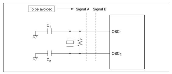
Figure 4.5 Board Design of Oscillator Circuit
