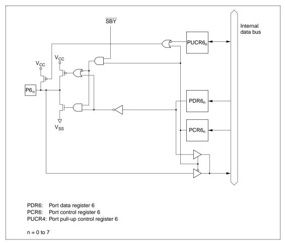
Figure C.6 Port 6 Block Diagram
